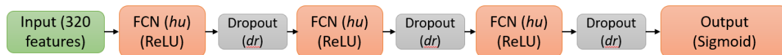
Figure 37. Visual representation of MLPNN classifier. The MLPNN architecture consists of three fully-connected hidden layers with hidden units hu and the ReLU activation, each followed by a dropout layer with a dropout rate dr .
